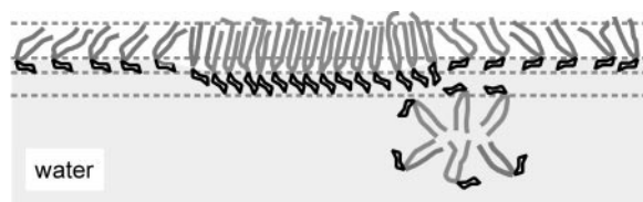
FIGURE 7 Molecular interpretation of the phase behavior of compressed HFA on pure water at 30°C. The monolayer is inhomogeneous with a higher-ordered phase forming on a micrometer scale. The micelles grow into the subphase rather than into the air.
